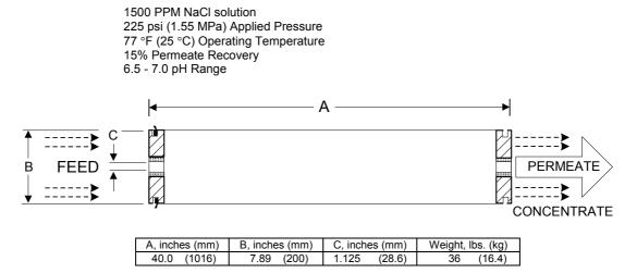
Notice: Permeate flow for individual elements may vary ±15 percent. Membrane active area may vary ±/.4%. Element weight may vary. All membrane elements are supplied with a brine seal, interconnector, and o-rings. Elements are enclosed in a sealed polyethylene bag containing less than 1.0% sodium meta-bisulfite solution, and then packaged in a cardboard box.
